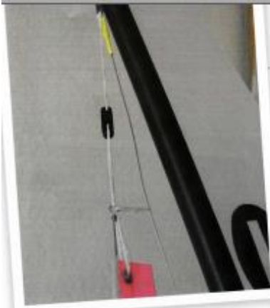
These head stay and leech lines should never be twisted
