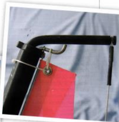
Align the head stay and backstay fittings
