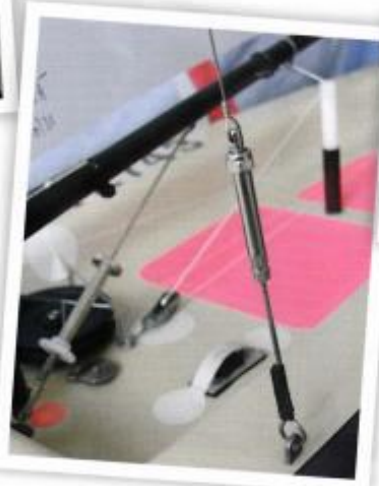
Side stay attachments. The bottom half permanently attached to the deck eye
